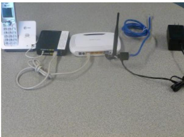
The image above shows an antenna power cord (Far Right) which connect in to a cable going to your dish (Right), a Wireless Router (Middle), a VoIP Phone Adapter (Left), and a regular wireless phone (Far Left). This is the setup for a wireless connection (If you have a dish on your building). Note: No Power cords are currently plugged in, and each device requires power to function correctly.
